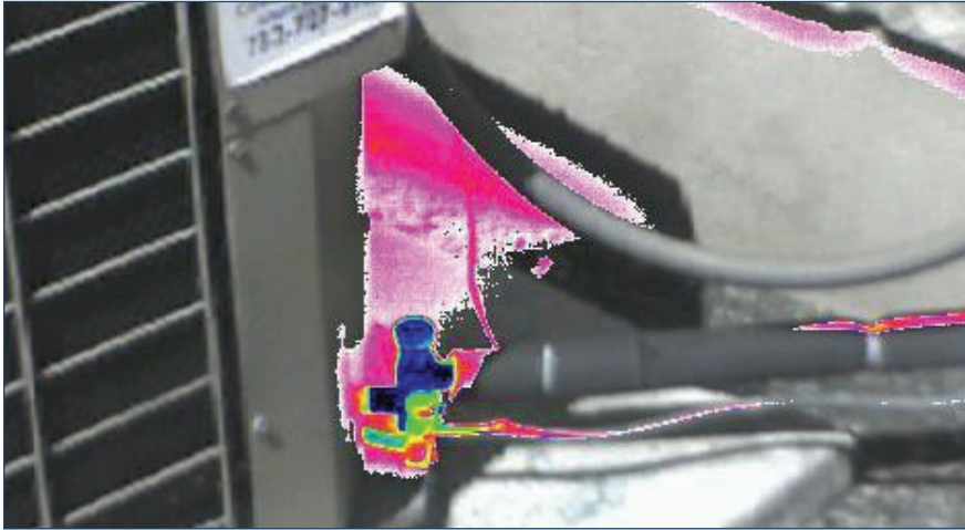
The CSI 9830 Fusion Mode reveals the infrared data over the visible image only in areas where temperatures fall within a customizable range.
