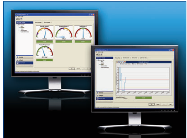
AMS Device Manager uses EDDL technology to create an asset dashboard with clear indication of device and asset status.
