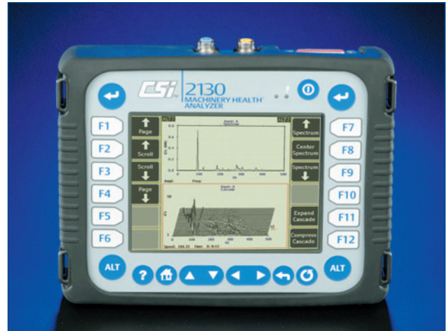
The Cascade application captures machine vibration during startup, coast-down, or over an extended period of time. Top half of screen shows spectra individually; bottom half of screen shows cascade plot.
